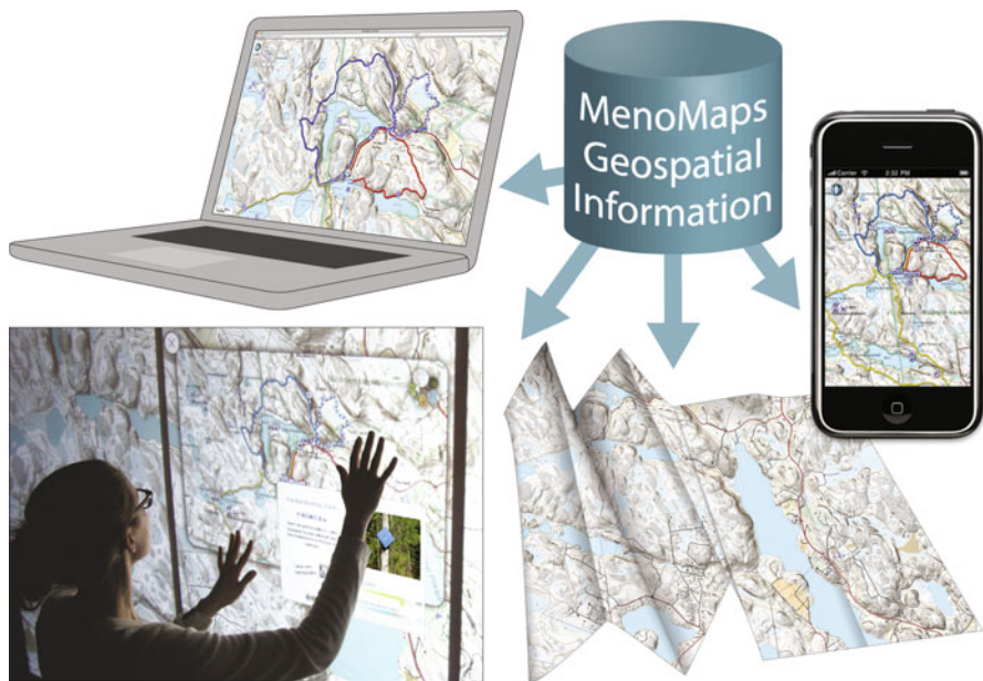
Fig. 12.1 The channels of the MenoMaps multipublishing service: the map applications for a mobile phone (iPhone) and a multi-touch screen, printed graphic maps and a web map (Flink et al., 2011). The data for all the channels is derived from the same data core
