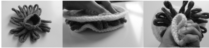
Fig. 9 Form iteration 3: A tentacle-like form was introduced, that could act as a pressure sensor between the two circular layers. It added an interesting visual and tactile quality to the interactions. However the two actions of flipping and squeezing were felt to be not so coherent. We decided to shift our focus back the flipping action.
