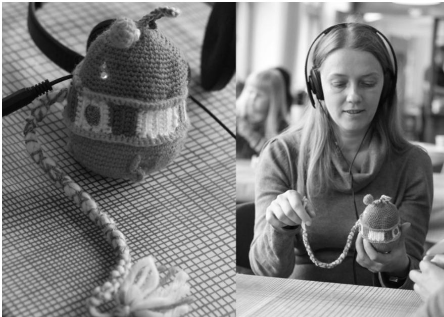
Fig. 3 The Soft radio: A crocheted radio that uses textile interactions of wrapping and twisting for operating the radio. Video available at http://narrativize.net/sofradio/
