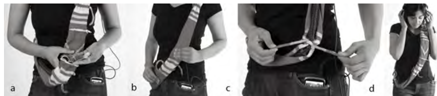
Fig. 2 The Music Sleeve: a) An opening that allows coins to be dropped into the sleeve. b) The sleeve is worn across one's shoulders, rotating the sleeve moves the coins within. c) The movement of the coins can be obstructed by tying the string. d) The music player on the phone is wirelessly controlled. Video available at http://narrativize.net/66/
