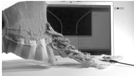
Fig. 15 Shape sensor: Three conductive rows on the knitted tube act as analog sensors detecting the shape of the stretched tube.
