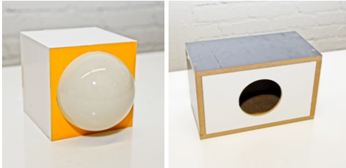
Figure 3. A cardboard mock-up of the convex display (left) and MDF construction mock-up (right) of 'Hole in Space'.
